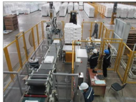
Manual Handling Eliminated using a new robotic palletizer
